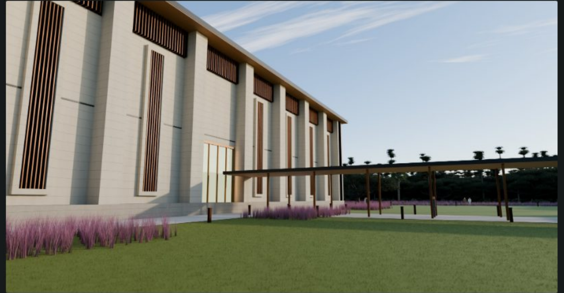
Proposed Project Tabby. Tabby-finish precast panels with oyster-shell aggregate, the same lifts and color.
